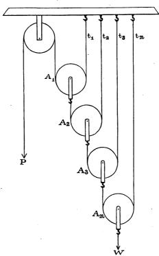
$A_s$ , ...  $A_n$  respectively, and  $t_1$ ,  $t_3$ ,  $t_4$ , ...  $t_n$  the tensions of the cords passing round these pulleys; then the pulley  $A_t$  is acted
